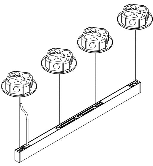
Follow steps 1-10 to mount the additional runs in the fixture. Fixture must be hung level at the desired height. If fixture is not level, light leaks may occur at the seam.
