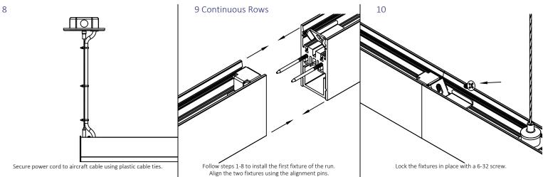
NOTE: JUNCTION BOXES MUST BE SOLIDLY FIXED TO THE CEILING AND ATTACHED TO THE STRUCTURAL MEMBER INSIDE THE CEILING BEFORE PROCEEDING WITH INSTALLATION.
