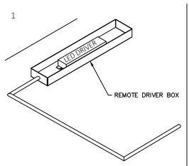
Install the remote driver box above the ceiling and run conduit that is not longer than 30ft in length from the fixture. Note: Use whip or plenum rated wires from the junction box to the remote box.
