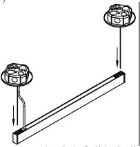
Insert the aircraft cable into the cable grippers on both sides of the fixture. Adjust the aircraft cables until the desired height is achieved. Note: Fixture must be level.
