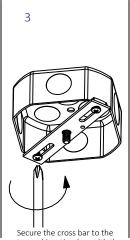
octagonal junction box with the junction box screws.
