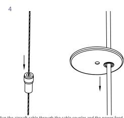
Run the aircraft cable through the cable coupler and the power feed cable through the canopy respectively.
