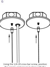
the canopy and secure in place with the cable coupler
