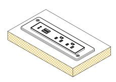
Step 3: Tighten screws to lock outlet in place.
