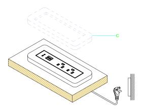
Step 4: Attach the cover; Connect to power supply.
