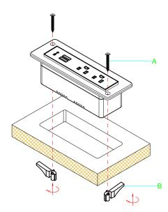
Step 2: Insert outlet from top,place the retaining clips over the threaded studs.
