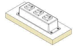
Step 3: Tighten screws to lock outlet in place.
