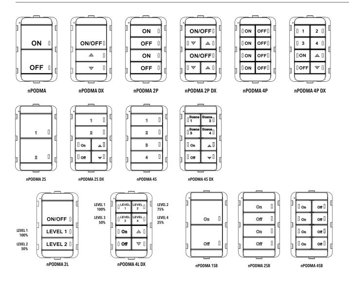
Dynamic wallpods below are paired with Acuity Brands nTUNE fixtures for out-of-box operation. Reference fixture cut sheets for additional details.
